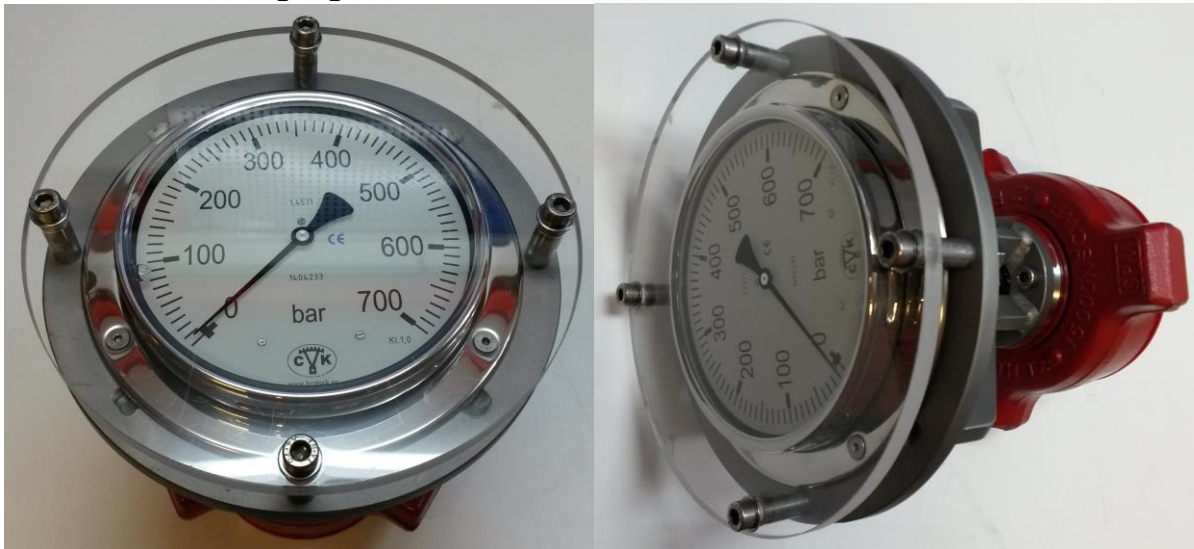
Figure 9 & 10 Pressure Gauge unit with 0-700Bar scale
